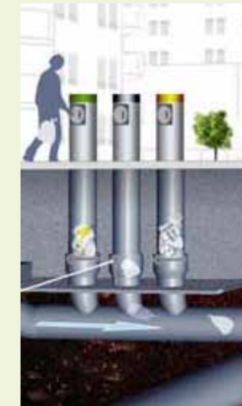
From the house to the waste removal system. Pneumatic waste systems like the one in this picture are especially suitable for use in ancient, crowded urban areas.
